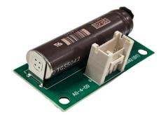
The AG-4-CO-M5042 is an embedded type module equipped with the Figaro's carbon monoxide gas sensor TGS5042, for accurately detecting carbon monoxide (CO) gas concentrations in various environments. The module has been precalibrated before leaving the factory and has good stability and selectivity. It allows users to easily and quickly integrate the module into various systems.
